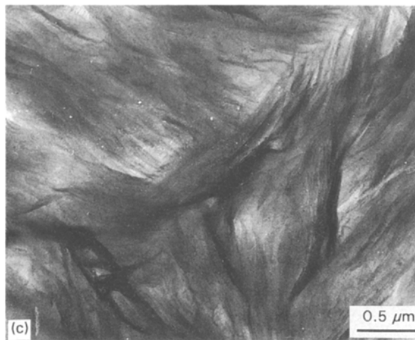
Figure 4 BF electron micrographs of HDPE-iPP multilayered films, heat treated at 150 °C for 10 min and then cooled slowly (at a rate of 0.5^\circ\text{C min}^{-1} ) to room temperature. The thickness of the HDPE layer is (a) 60, (b) 120, and (c) 150 nm, respectively.
